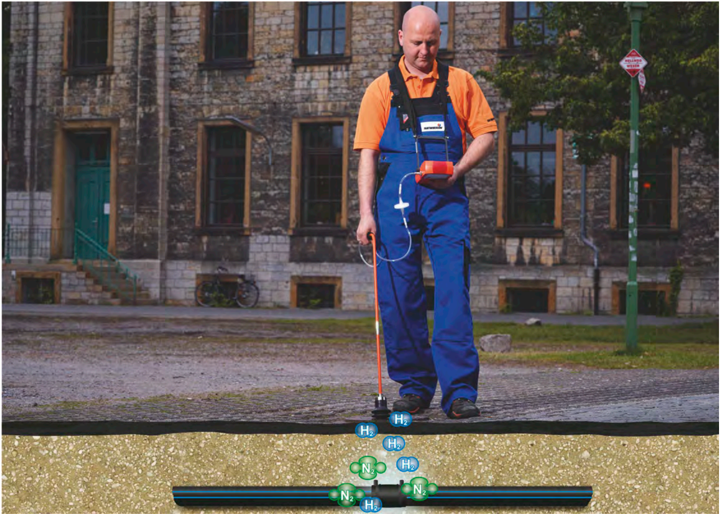
Figure 4: Tracer gas to pinpoint leaks in water pipes
