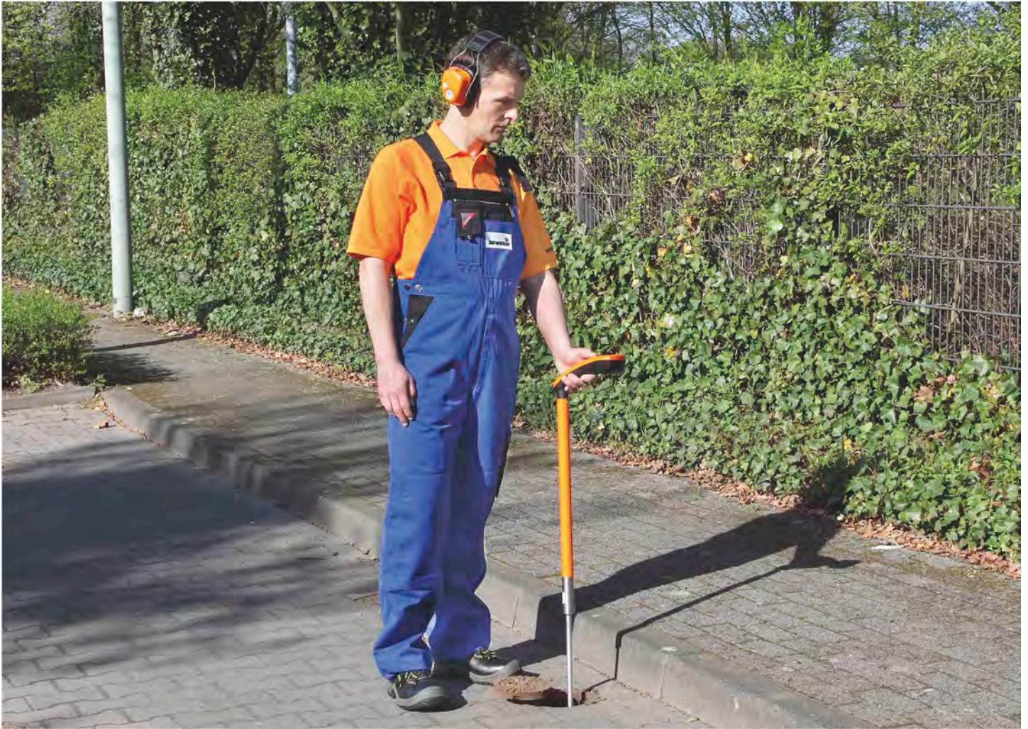
Figure 2: Using a test rod for prelocation
