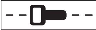
Fig. 27: Receiver oriented to the assumed route of the line for passive location
