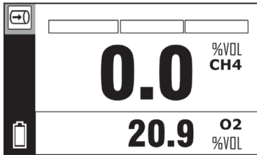
Fig. 24: Measuring mode ( here: Measuring application ) top left (information area): Symbol of the current application
