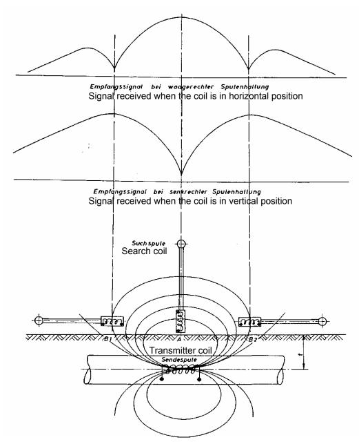
Fig. 3: Determination of location and depth based on the field-line trend:
