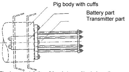
Fig. 1: Installation of the pig transmitter (schematic representation). The transmitter part remains free.
